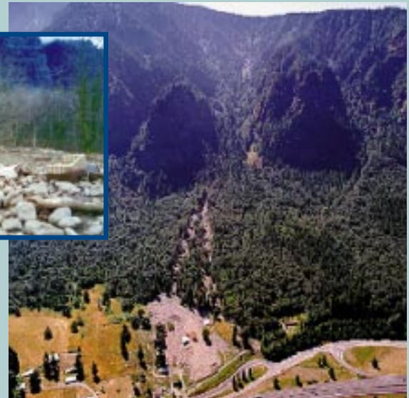
This debris flow occurred in the Columbia River gorge near the town of Dodson, Oregon, during a rainfall and snowmelt event in February 1996 (Photo Inset: S. Cannon, USGS). The combination of rainfall and snowmelt resulted in severe flooding and landsliding throughout the Pacific Northwest. The debris flow shown here was deposited in a number of separate events over a period of 2 days. The flows originated high on the palisade and traveled through the steep canyon. The occupants of the house escaped with their lives when they heard a loud rumbling and crashing of trees and saw the approaching material through their kitchen window. Boulders, mud, and debris from these and several nearby debris flows were deposited across the east-bound lanes of Interstate Highway 84, and blocked the highway for 5 days (Aerial Photo: D. Wieprecht, USGS).
